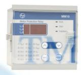
**Motor Protection Relay;** These Motor Protection Relay's have designed for the protection and active security of medium and large size induction motors. The relay also computes the positive (Id) and negative (Is) sequence components of phase-current system. The earth current input circuit includes a 3rd harmonic active filter.
