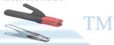
**Electrode Holders;** These are fully insulated electrode holders which conform to ISI Standards (IS-2641). Its handle, lever, spatter protection guards are made of fire retardant and heat resistant imported material. Special quality of copper alloy as main conductor & brass jaws ensure good contact with electrode and continuous duty cycle. This holder is very light weight and suitable for cables up to Al120/Cu70 sq.mm.
