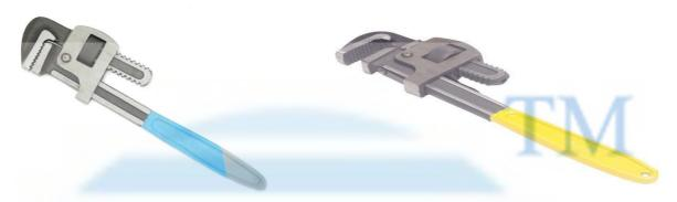
**PIPE WRENCH:** We deals with Taparia make Heavy Duty Pipe Wrench has drop jaws forged from chrome molybdenum [Cr Mo] steel. It comes with extremely precise machined jaw teeth with appropriate teeth angle of 76° to enables positive grip on the job. Differential hardening of Teeth and Body of the Jaw enables high torque and high wear resistance of the Jaw.
