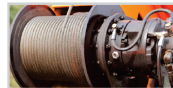
Hydraulic Winch (Reputed make) High on performance & low on maintenance. 6 fall snatch block with line pull of 2.5 T.
