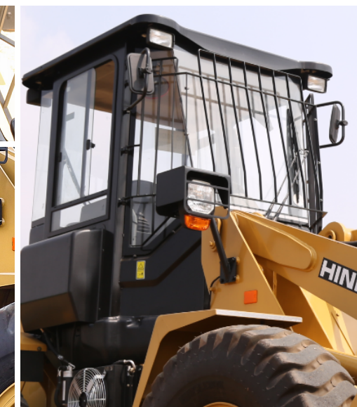
Guards – Windshield & Lights, Work light front
